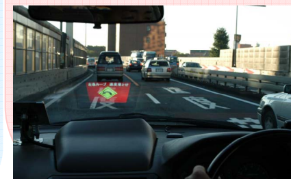
Testing a curve entry warning system (Sangubashi, Metropolitan Expressway)
