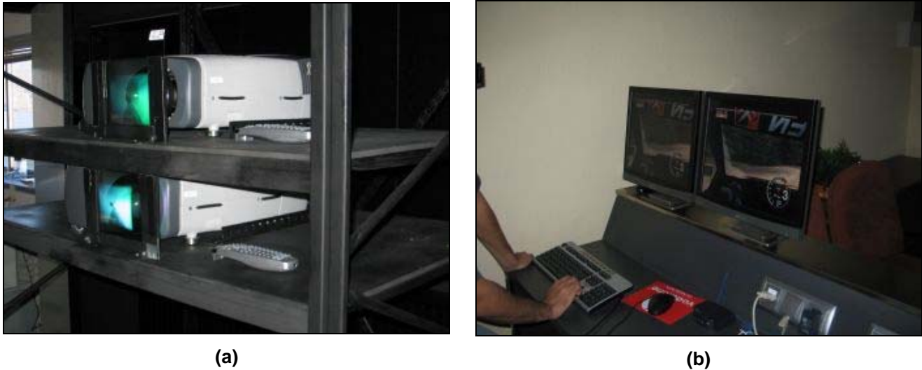
Figure 8: Stereo projection system (a) and their output monitors (b)
