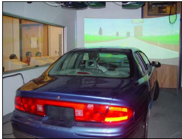
Figure 1: A driving simulator at the Virginia Campus of The George Washington University [2]
